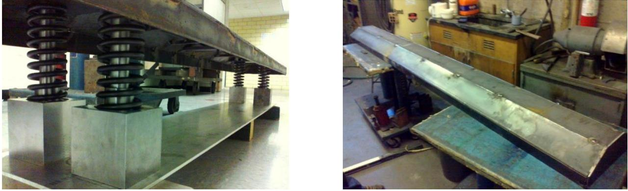
Figure 3. Speed bump cover unit fabricated. Left: linear bearing, springs and mounting arrangements. Right: fabricated speed bump cover
